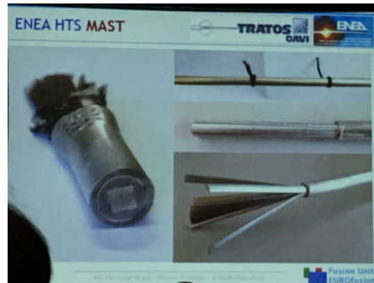
Various types of REBCO conductor for high current using ROEBEL and CORC conductors
