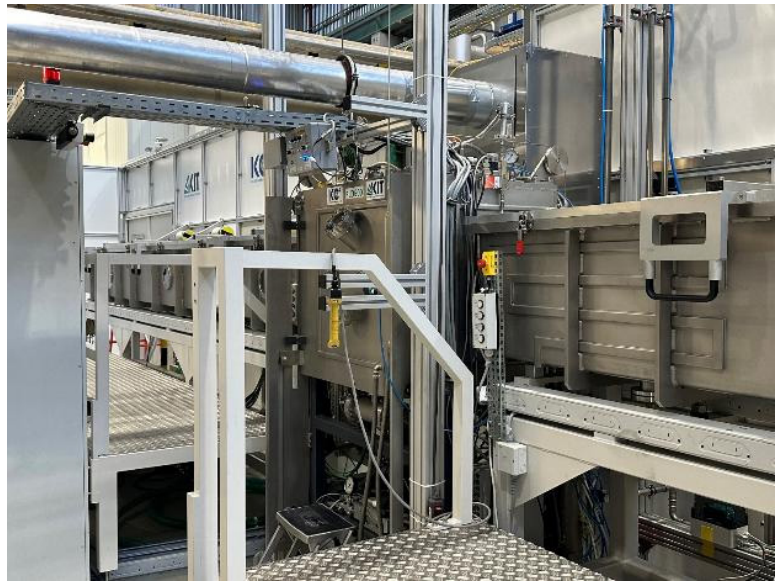
Pictured is an HTS coated conductor (CC) manufacturing line at KIT Campus North based on Bruker's manufacturing techniques for long CC and wide tapes.
