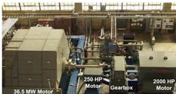
FIGURE 8. THIS 36.5 MW SHIP PROPULSION MOTOR EMPLOYS HTS FIELD WINDING. PHOTO COURTESY OF AMSC.
