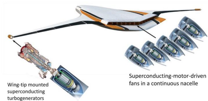
FIGURE 7. A TURBOELECTRIC PROPULSION SYSTEM REDUCES FUEL USAGE WITHOUT COMPROMISING PERFORMANCE. THE REQUIRED ELECTRICAL MACHINES ARE SHOWN IN THE SCHEMATIC ABOVE. IMAGE COURTESY OF THE UNITED STATES NATIONAL AERONAUTICS AND SPACE ADMINISTRATION.
