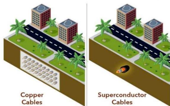
*Figure 1 Superconducting cables can replace many conventional copper cables and transfer transmission power at distribution voltages.*
