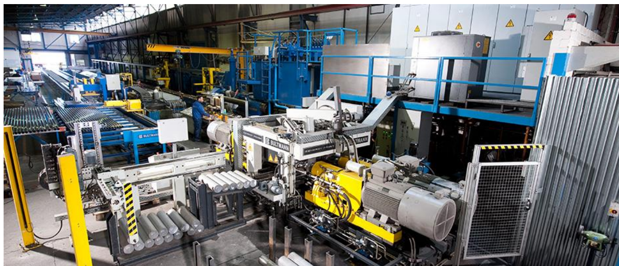
Figure 8. Bültmann magnetic billet induction heater installed at Weseralu in Minden, Germany. Photo courtesy of Bültmann.
